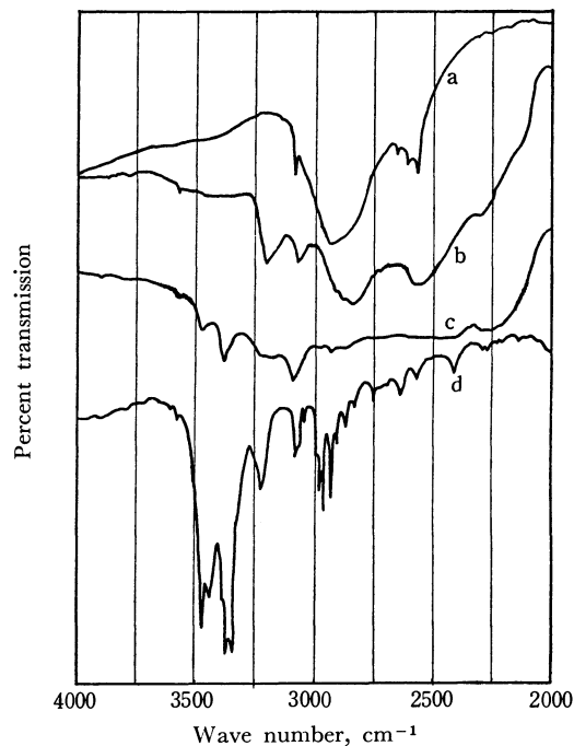
Fig. 6. Vibrational spectra, a) 3-nitro-4-methylaniline hydrochloride, b) the solid 3-nitro-4-methylaniline-picric acid, c) the same in the molten state, and d) the amine.
