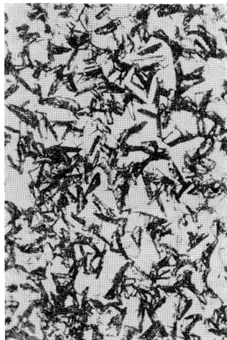
Fig. 6. Phosphate coating on buff-polished iron. (5 min, \times 160 ) Cathodic current 3 mA/cm 2 , without rotation.
