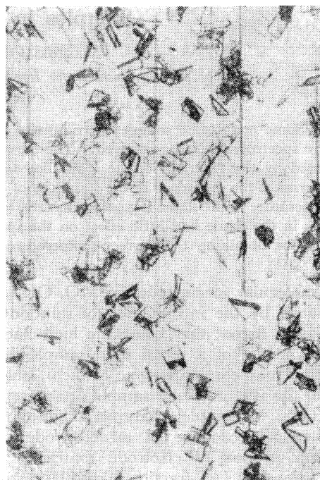
Fig. 7. Phosphate coating on buff-polished iron. (5 min, \times 160 ) Without cathodic current and rotation.
